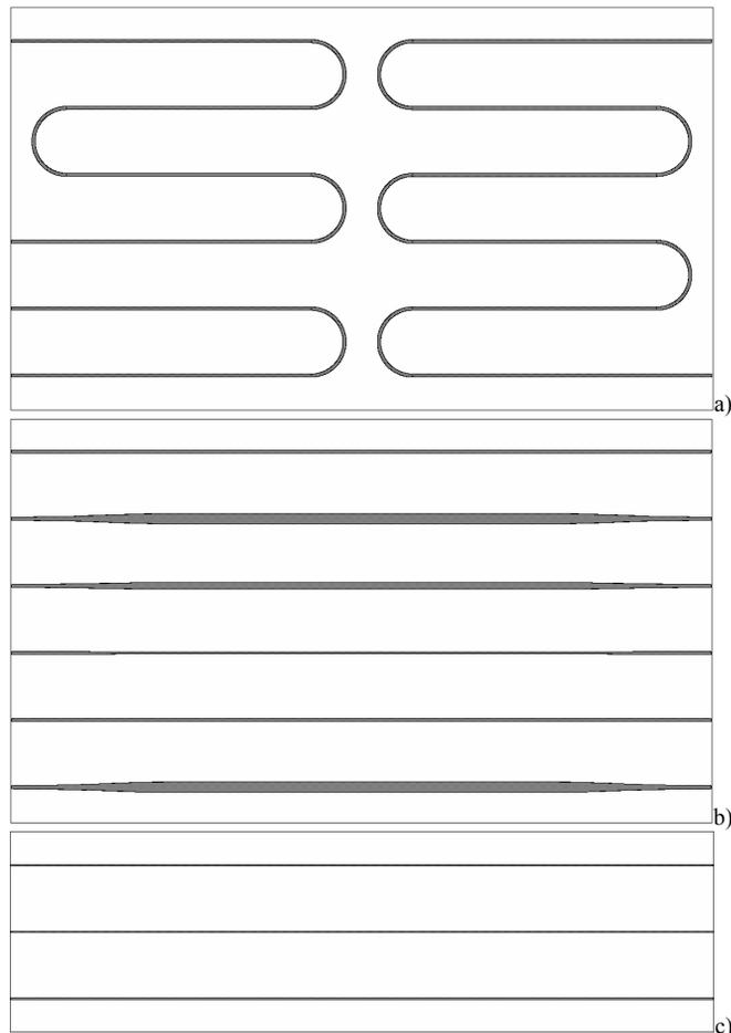
Fig. 1. Plan view of the board with printed microstrip traces: a) uniform meandered lines (Boards 1, 2); b) traces with different width (Boards 3, 4); c) straight uniform lines for PIM3 characterisation of different PCB laminate compositions (Boards 5 - 10).
