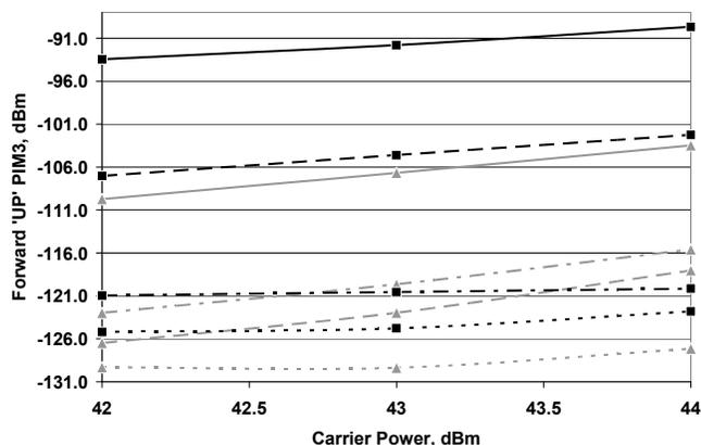
Fig. 7. Forward ‘UP’ PIM3 dependence on carrier power in GSM 900 band. Black squares – Board 1: dotted line – residual PIM3 (SLOPE=1.19:1); dash – 917mm (SLOPE=0.40:1); dash-dot – 1828mm (SLOPE=2.39:1); solid – 2736mm (SLOPE=1.89:1). Grey triangles – Board 2: dotted line – residual PIM3 (SLOPE=1.08:1); dash – 917mm (SLOPE=4.22:1); dash-dot – 1828mm (SLOPE=3.13:1); solid – 2736mm (SLOPE=3.69:1).
