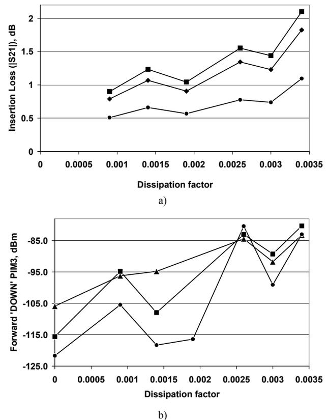
Fig. 5. Insertion loss ( $|S_{21}|$ ) (a) and forward 'DOWN' PIM3 (b) at 2×43 input power in GSM 900 (dots), DCS 1800 (squares) and UMTS 1900 (triangles) bands vs. dielectric dissipation factors of the substrates specified in Table I.
