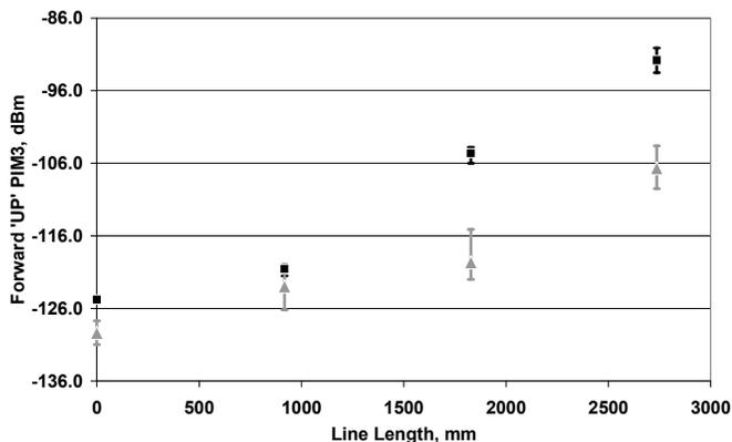
Fig. 3. Forward PIM3 vs. line length at  $2 \times 43$ dBm carrier power in GSM 900 band averaged over the swept frequency band 910-915MHz: black squares – samples on the Board 1; grey triangles – samples on the Board 2.
