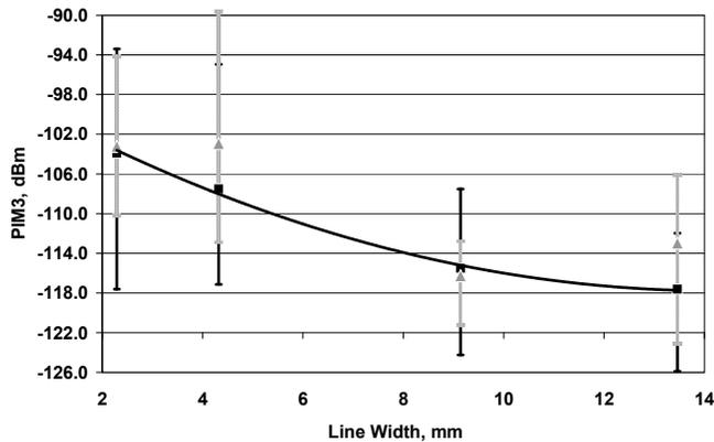
Fig. 4. Forward 'UP' (black squares) and reverse 'UP' (grey triangles) PIM3 vs. the microstrip line width in GSM 900 frequency band.
