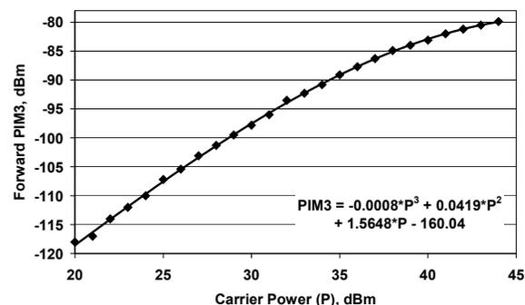
Fig. 6. Forward PIM3 dependence on the carrier power for a microstrip line on the Board 7 at 910MHz PIM3 frequency (PIM3 measurements in time)
