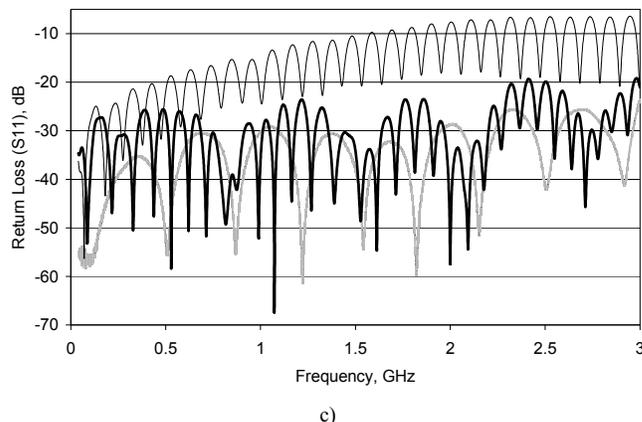
Fig. 2. Comparison of two types of board launchers: (a) – direct cable launcher, (b) – edge-mount DIN7/16 launcher; and (c) - typical RL measured on Board 7 (bold solid line – direct cable launcher, thin solid line – edge-mount connector, dotted line – the original cable assembly).
